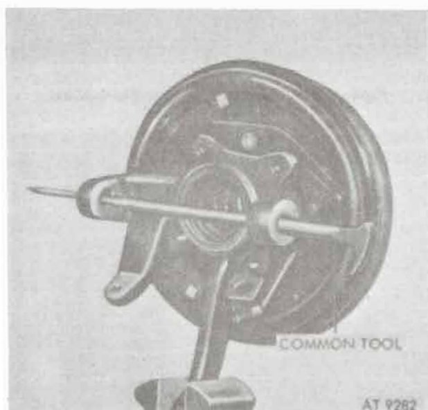
Figure 10-42. Securing drive flange from turning.
