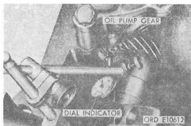
Figure 4-254. Measuring oil pump gear backlash.
