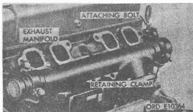
Figure 4-77. Exhaust manifold attaching parts.
