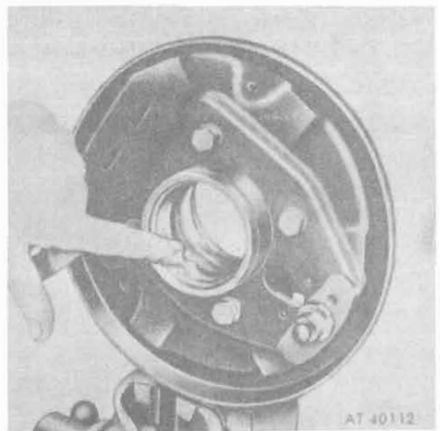
Figure 10-59. Coating bearing cups in with grease (GAA).
