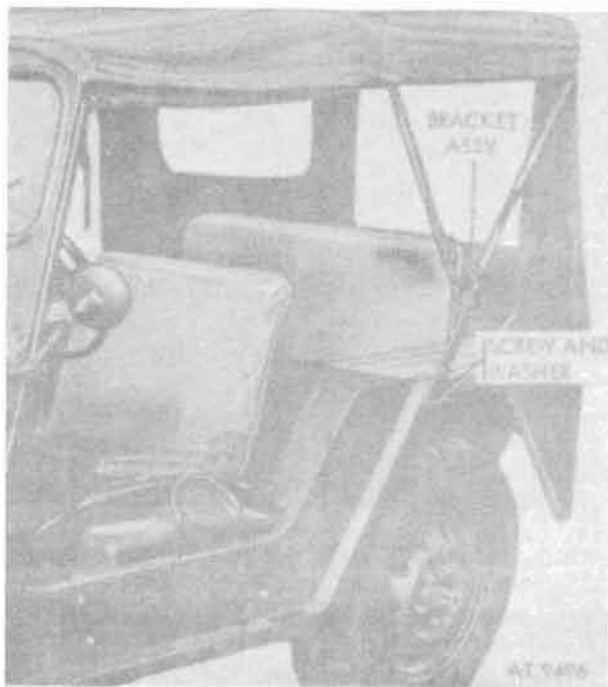
Figure 18-75. Removal of soft top bows and brackets.
