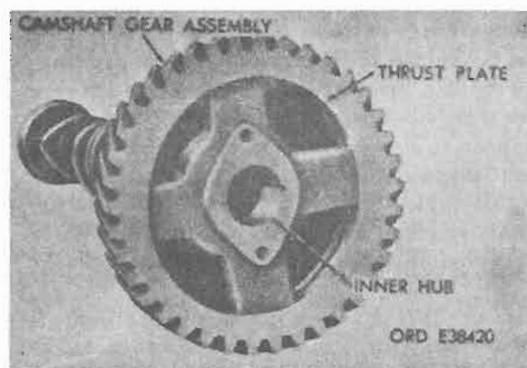
Figure 4-177. Camshaft gear installation.
