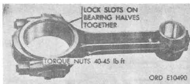
Figure 4-164. Connecting rod assembly.
