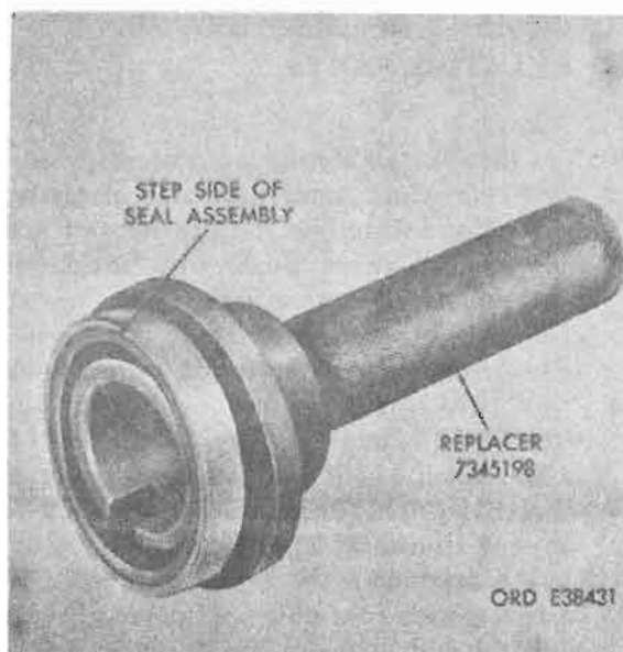
Figure 4-195. Oil seal assembly installation on replacer tool, 7345198.
