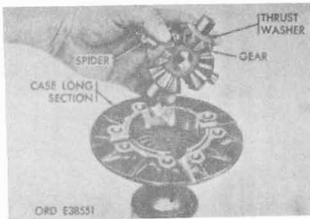
Figure 12-30. Differential spider, spider gears, and thrust washers.
