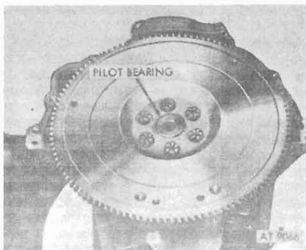
Figure 4-248. Clutch pilot bearing installation.
